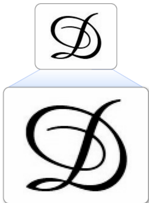
ClearType with y-direction antialiasing smooths out the jagged edges on shallow curves and other y-direction features
