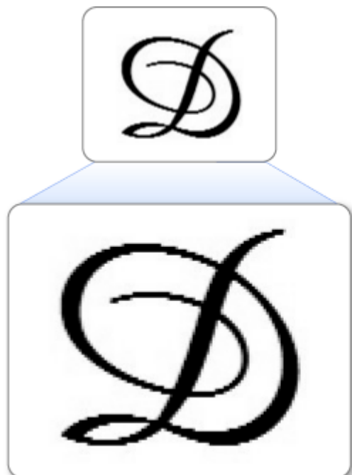
Enlarged view of Capitol Script D shows jagged edges on shallow curves
